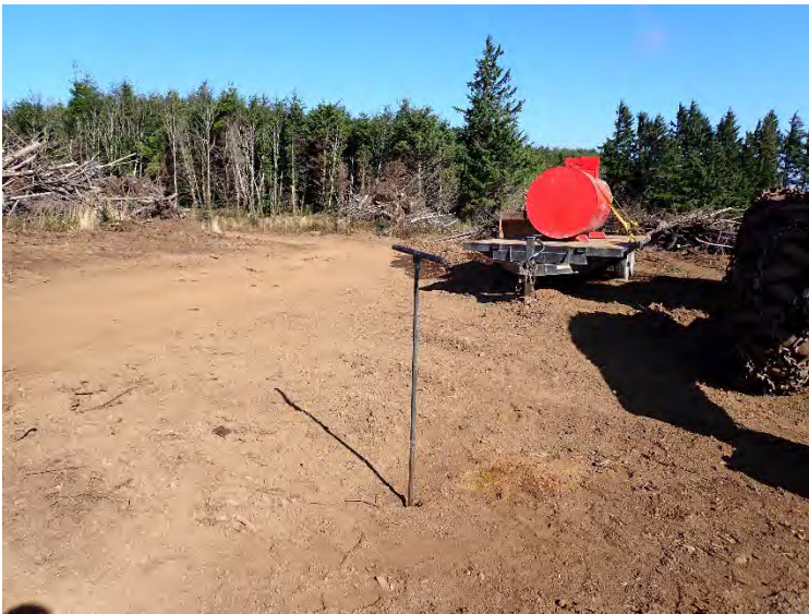
Hand auger boring 1 near proposed shop site.
